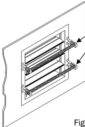
Probes supplied are 2 in. [50.8 mm] longer than the specified opening size to allow for bracket installation and damper blade clearance.
