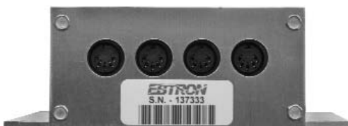
Accepts 4 probes, 1 sensor each.
