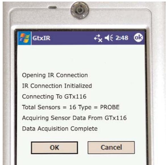
Figure 23. Typical PDA Display of *EB-Link* Initial Data Acquisition Screen
