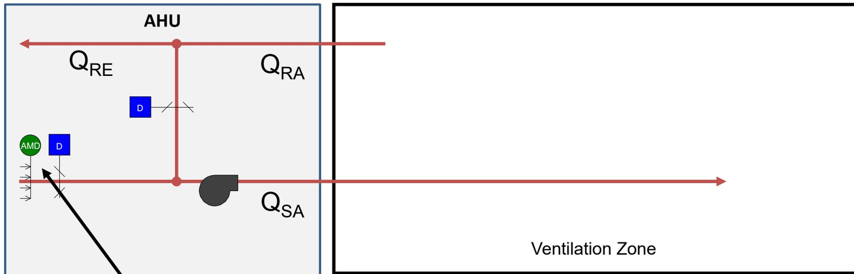
High Sensor Density Thermal Dispersion AMD (i.e. EBTRON GTx116e-PC or GTx116e-P+)
