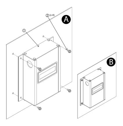
Step 1. Locate a position for the transmitter so that the connecting cables from all of the sensor probes will reach the receptacles on the bottom of the transmitter enclosure.
