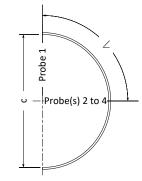
If the probes were ordered for a duct with internal insulation, use the external diameter of the duct for 'c' to calculate 'b'.
