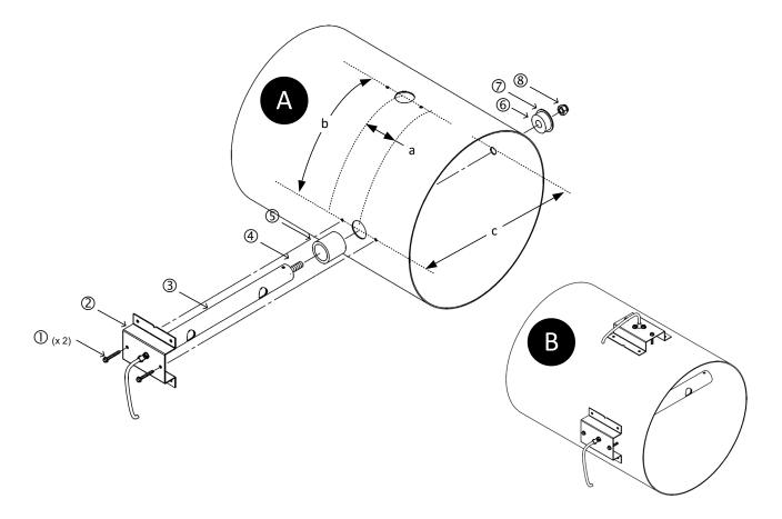
Step 1. Select a location in the duct or plenum opening that meets or exceeds EBTRON's recommended placement guidelines.
